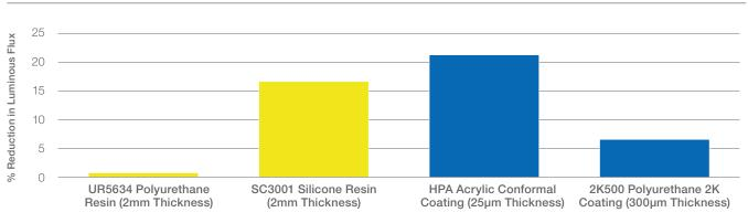
Protection Media Applied at Typical Application Thickness
